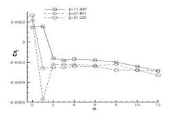
Figure 16. The stability derivative  $Cn_{\beta}$  vs. AOA at three different  $\beta$ .
