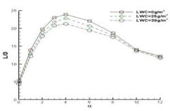
Figure 19. The lift to drag ratio vs. AOA at different rain rates.
