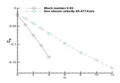
Figure 10. The pitching moment coefficient  $C_{\rm M}$  vs. AOA at two different velocities.
