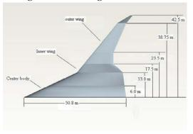
Figure 2. Blended Wing Body geometry model. 12
