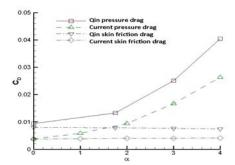
Figure 9. Pressure drag and skin fraction drag comparison.
