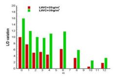
Figure 20. The lift to drag ratio vs. AOA comparison at two rain rates.
