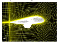
Figure 4. Near mesh of the Blended Wing Body.
