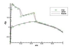
Figure 7. M6 Cp distribution at section y/b=0.65.
