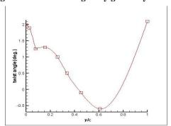
Figure 3. Twist angle distribution.
