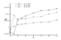
Figure 14. The stability derivative  $\operatorname{Cl}_\beta$  vs. AOA at three different  $\beta$ .
